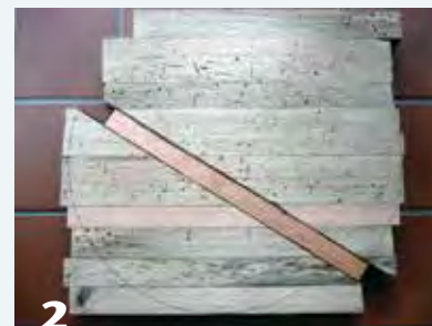
After the initial, parallel glue-up, the blank is cut at an angle and an additional piece glued in.
