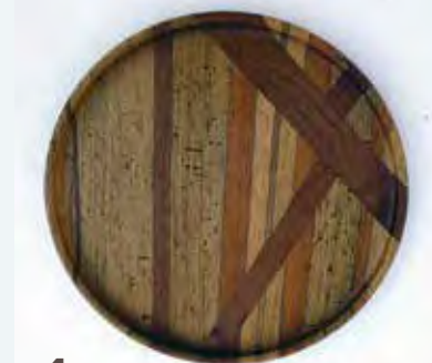
This design required two angled cuts after the initial parallel glue-up. A glueblock was used for turning a tenon, so the piece could be held in a scroll chuck.
