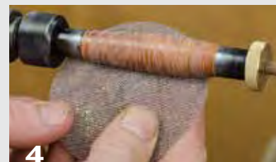
4 Finish the finish with Abranet. The high spots show up as opaque streaks. Aim for a uniformly opaque surface, which is then polished with increasingly finer abrasives.
