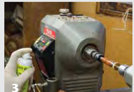
3 A blast of aerosol accelerator readies the turning for the next coat of CA. Use plenty of ventilation.
