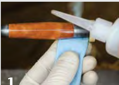
1 The objective is to apply the CA quickly in a single traverse. CA adheres poorly to metal, so a little contact with the bushings is not a problem.
